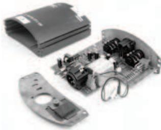
*Front and back panels screw to an aluminum channel. The PCB is supported by the jacks. A hit to the panels is transferred directly to the PCB. The switch and jacks are unprotected.*
