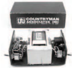
*Front and back panels are integrated to a slide-in-frame. Switch and jacks are recessed for protection. PCB is encased in epoxy making repair impossible.*
