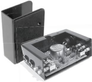
*Radial DI's feature steel I-beam internal construction for maximum strength. The outer metal wrapper uses bookend design which creates an overhang that protects the switches and jacks. The PCB is supported with four welded stand-offs to reduce stress on the PCB. A rubber pad covers the bottom for electrical isolation and helps the DI 'stay put' on top of amps.*
